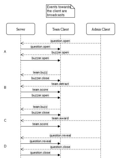
The above diagram shows how the protocol works. It has four major parts: Opening the question (A), Starting and stopping the buzzer (B), correctly answering the question (C), and clean up (D).
