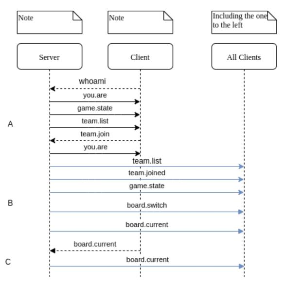
The above diagram represents the protocol for joining a game (A), the game starting (B), and the client requesting an update of the board (C). There is a bit of individual client housekeeping housekeeping at the start, and then most of the communication from the server to the clients is in broadcast form.
